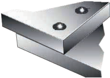
Plug Welds (Fig 1-19j)
